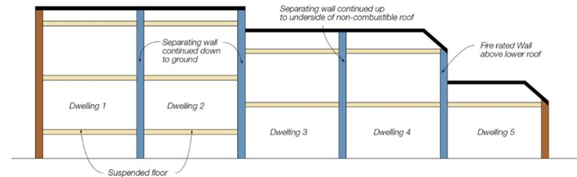
Where the internal fire separation wall extends beyond the roof line on one side only and becomes an external wall, contact Hebel Technical Services for advice on PowerPanel<sup>XL</sup> and PowerPanel<sup>50</sup> external wall solutions.
