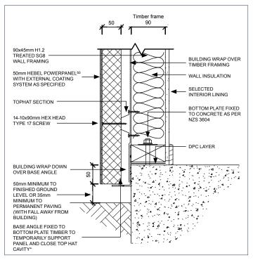
\*NOTE : THIS BASE ANGLE DETAIL IS NOT APPLICABLE FOR A FIRE RATED WALL- SEE SECTION 2.2
