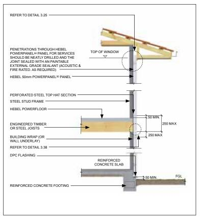
NOTE: These gap widths can be reduced for low shrinkage floor systems. Contact the floor system manufacturer for guidance on acceptable gap width. Refer also to NZS 3604: 2011
