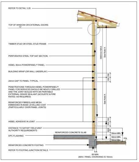
NOTE A: Panel length to be selected from available panel lengths as set in section 1.4 - 'System components' of this guide. \* Denotes horizontally aligned 50mm PowerPanel<sup>50</sup> panel
