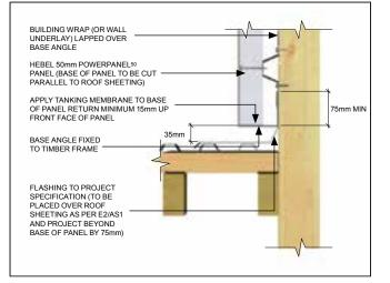
Detail 3.27 – Typical roof/parapet wall detail
