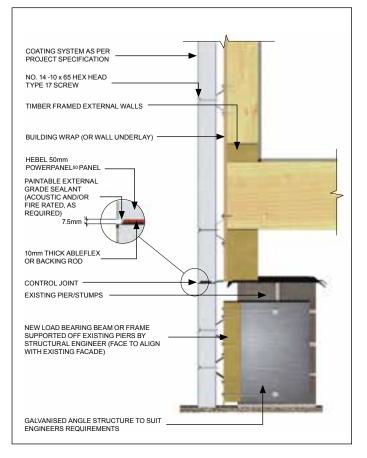
Detail 3.23 - Base detail suspended floor - pier connection
