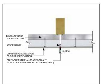
Detail 3.40 – Horizontal control joint – brick veneer to Hebel PowerPanel<sup>50</sup> Panel
