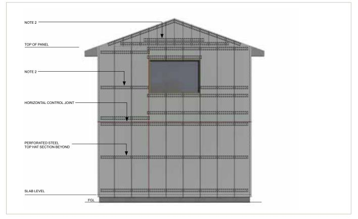
NOTE 1. Number of Top Hats and Top Hat spacing to be confirmed by the building designer. 2. Additional Top Hats may be required, for suspended panels. Refer to tables 1.7 - 1.10 on page 11 for number of Top Hats required (or Tables 2.3 - 2.6 on Page 20 for Boundary Walls) 3. These details have not shown the set-out of Top Hats to accommodate control joint locations. This is the responsibility of the building designer.
