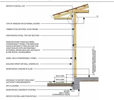
Detail 3.6 - Single storey construction - high wall section detail - (3900mm MAX)
