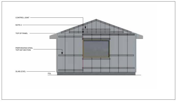
NOTE 1. Number of Top Hats and Top Hat spacing to be confirmed by the building designer. 2. Additional Top Hats may be required, for suspended panels. Refer to tables 1.7 - 1.10 on page 11 for number of Top Hats required (or Tables 2.3 - 2.6 on Page 20 for Boundary Walls) 3. These details have not shown the set-out of Top Hats to accommodate control joint locations. This is the responsibility of the building designer.
