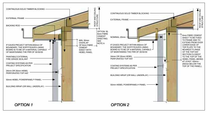
NOTE A: Where solid timber blocking is installed under the frame top plate (OPTION A) such blocking must extend below the level of the soffit lining. Where 6mm fibre cement sheeting is installed against the top plate against the top plate & studs, such lining should be overlapped a min. of 50mm with the Hebel external wall panel. (OPTION 1B).
