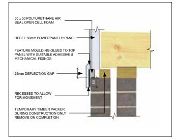
Detail 3.41 - Typical vertical control joint
