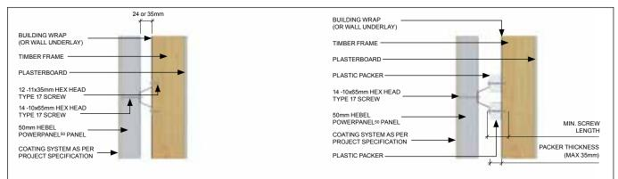
TYPICAL WALL FIXING DETAIL FROM OUTSIDE
