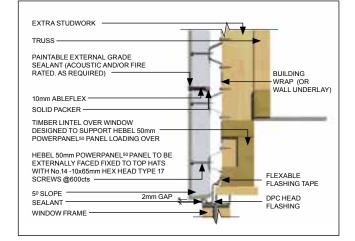
Detail 3.32 - Gable end wall detail - lintel panel over window
