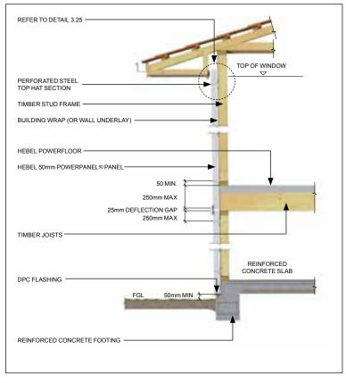
Detail 3.10 –Two storey construction – typical timber frame section using joists with >1% shrinkage
