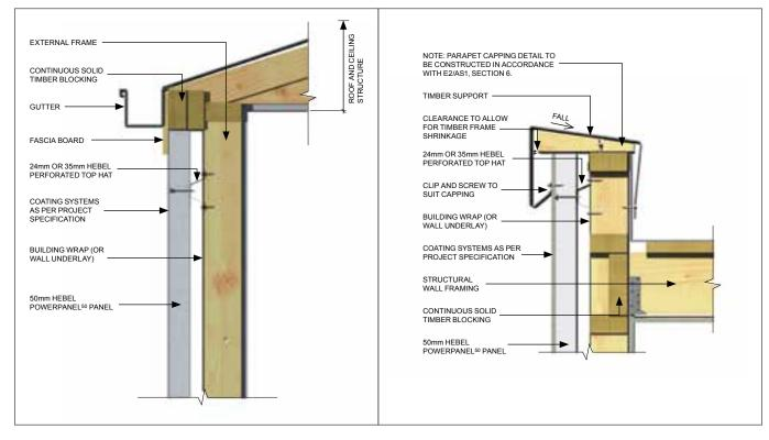
Fig. 2.4– 50mm PowerPanel<sup>50</sup> Boundary Wall - No Eaves Detail
