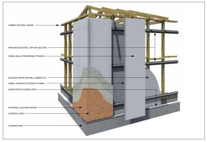
Fig. 1.1 – Typical Home Construction Application
