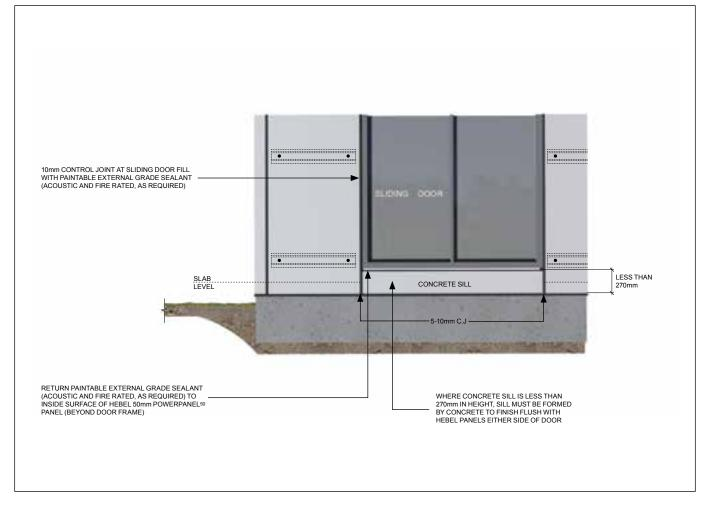
Detail 3.53 – Sliding door sill detail – option 2 - concrete sill >270mm
