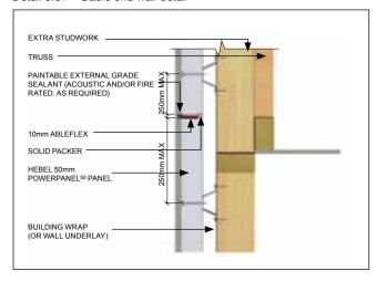
Detail 3.33 - Column Detail (Glued & Screwed)
