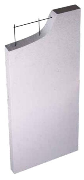
At the heart of the Hebel residential external wall system is the Hebel PowerPanel<sup>50</sup> - a 50mm thick, steel reinforced building panel made from AAC (Autoclaved Aerated Concrete) supplied in lengths of 2200mm to 3000mm with standard width of 600mm.
