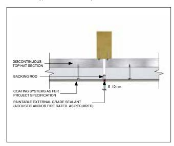
Detail 3.40 – Horizontal control joint – brick veneer to Hebel PowerPanel<sup>50</sup> Panel
