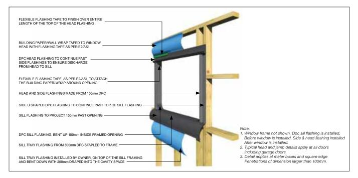
Detail 3.46 – Typical window sill detail – aluminium window frame - OPTION 1
