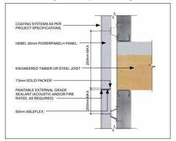
**NOTE:** The position of the horizontal control joint must be such that the panel must not cantilever more than 250mm past the last Top Hat, top and bottom. Top Hats must not be fixed to joists
