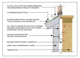
Detail 3.47 – Typical window sill detail – aluminium window frame - OPTION 2
