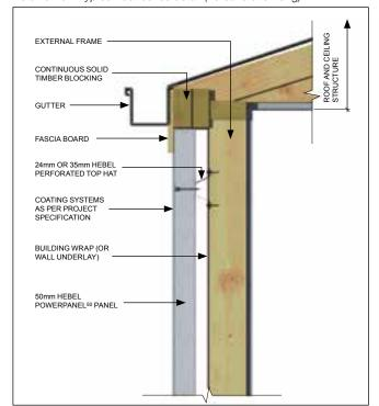
Detail 3.27 - Typical roof/parapet wall detail
