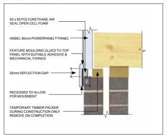
Detail 3.41 - Typical vertical control joint
