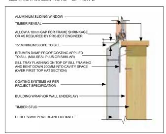
Detail 3.48a – typical window sill detail timber window sill joinery detail
