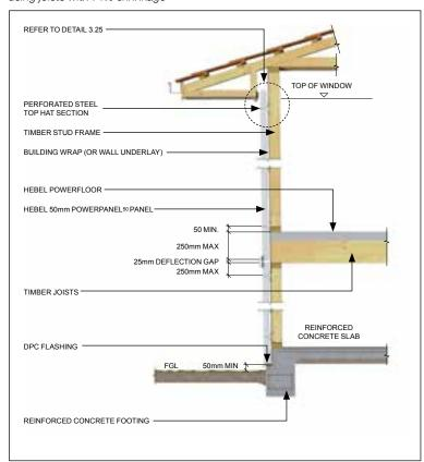
Detail 3.11 – Two storey construction – steel frame section or engineered joists with ≤1% shrinkage
