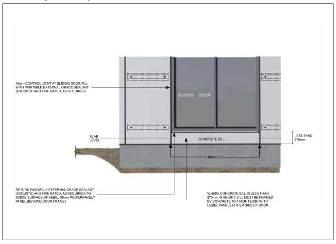
Detail 3.53 - Sliding door sill detail - option 2 - concrete sill >270mm
