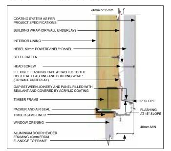
Detail 3.49a - Timber window head - joinery detail
