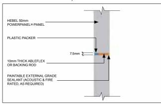
Top view - Horizontal control joint
