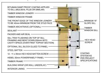
Detail 3.49 - Window header - alternative detail
