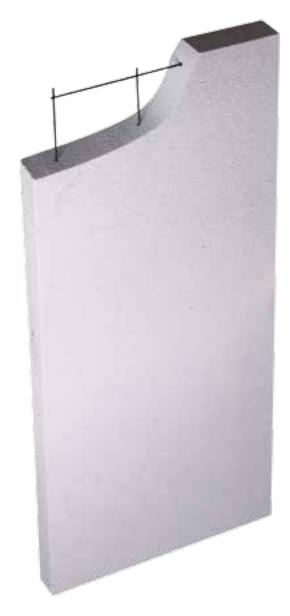
At the heart of the Hebel residential external wall system is the Hebel PowerPanel<sup>50</sup> - a 50mm thick, steel reinforced building panel made from AAC (Autoclaved Aerated Concrete) supplied in lengths of 2400mm and standard widths of 600mm.
