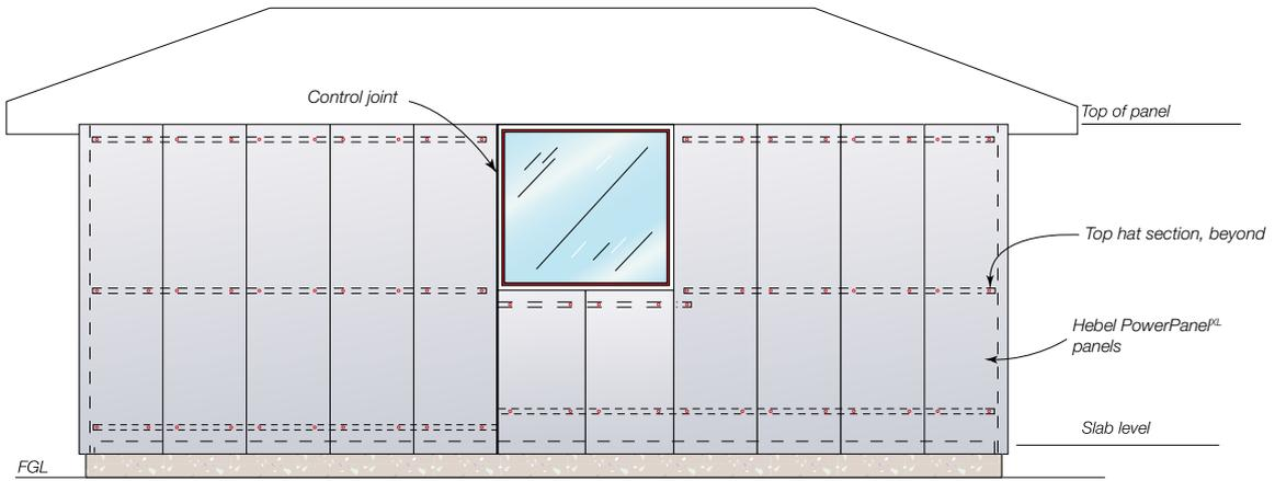
Figure 3.5.1.4 Single storey construction – gable end elevation
