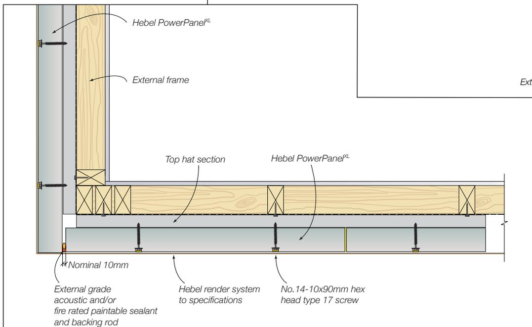
Figure 3.5.7.3 Typical detail for control joints positioned on corner
