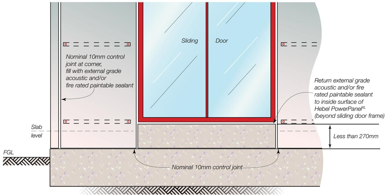
Figure 3.5.8.9 – Sliding door sill detail – section view – PowerPanel<sup>XL</sup> sill > 270mm
