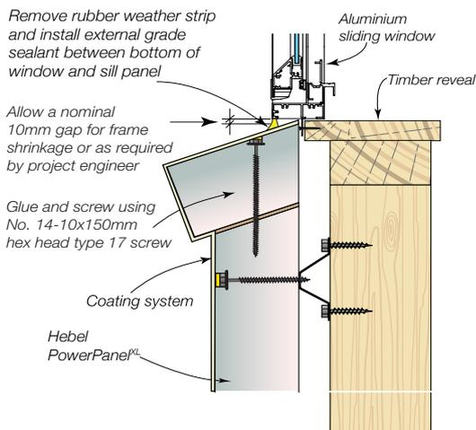
NOTE: Include suitable backing rod and sealant for 5-10mm gaps.
