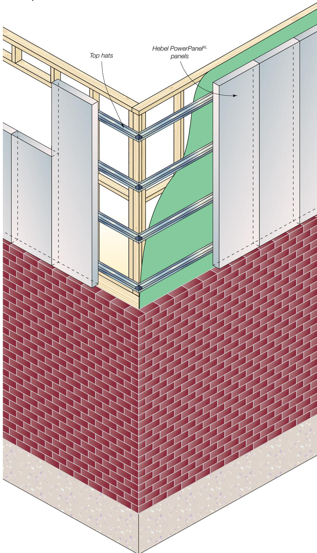
Figure 3.5.3.2 Two storey additions – typical section with brick veneer below
