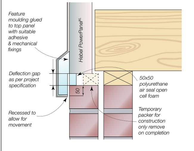
**Figure 3.5.7.8 Horizontal control joint – brick veneer to Hebel PowerPanel<sup>XL</sup>**
