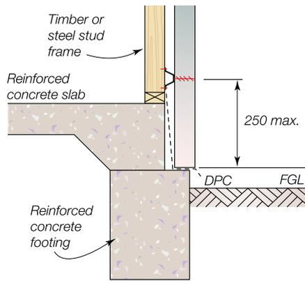
Figure 3.5.5.2 Junction to deep concrete edge beam
