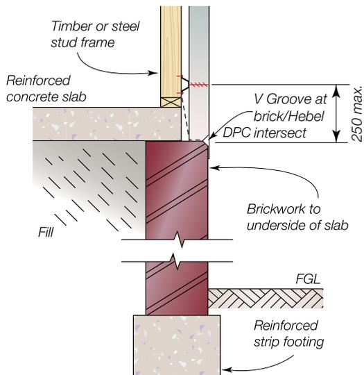
Figure 3.5.5.4 Junction to masonry dwarf wall
