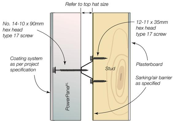
**Figure 3.5.4.2 Hebel PowerPanel<sup>XL</sup> Boundary Wall system fixing detail**
