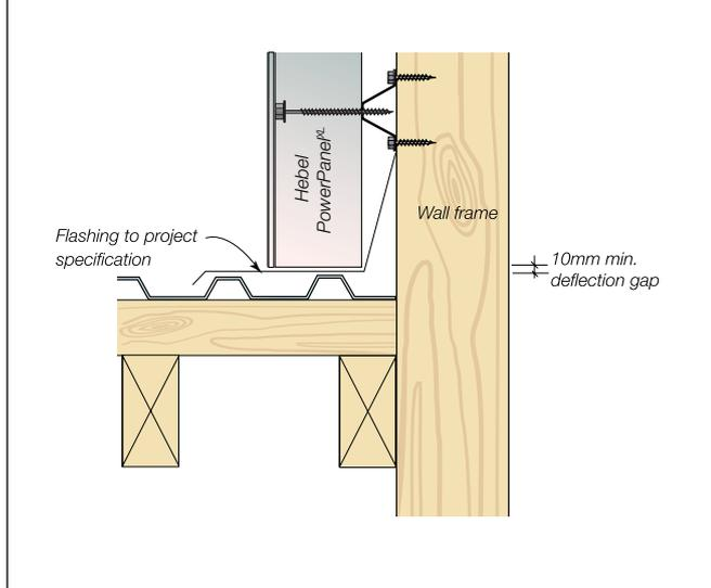
Figure 3.5.6.4 - Roof to wall junction detail - Option 2
