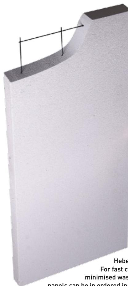
75mm steel reinforced Hebel PowerPanelXL. For fast construction with minimised waste, 600mm wide panels can be in ordered in stock lengths of 2400, 2550, 2700, 2800, 2850, 3000 and 3300mm.
