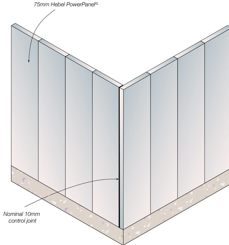
Figure 3.5.7.4 Typical detail for control joints positioned away from a corner
