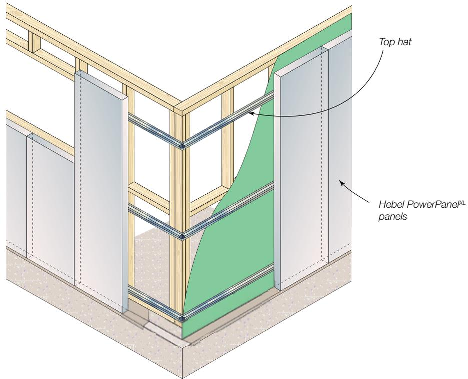
Figure 3.5.1.2 Single storey construction – isometric view detail panel suspended
