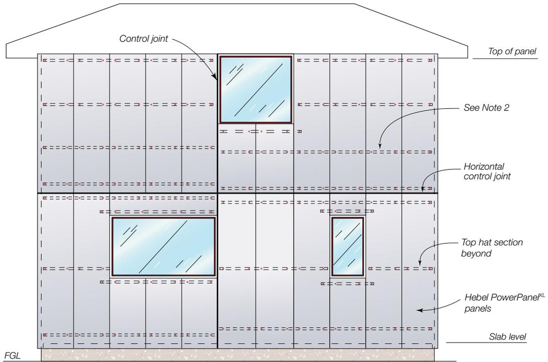
Figure 3.5.2.3 Two storey construction – gable end elevation
