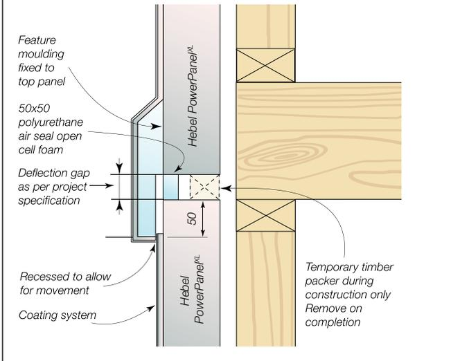
**Figure 3.5.7.6 Typical horizontal control joint steel stud frame or engineered timber joists  $\leq 1\%$  shrinkage**
