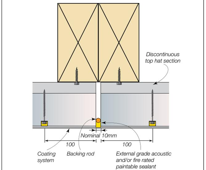
Figure 3.5.7.11 Control joint – discontinuous top hats on a single stud
