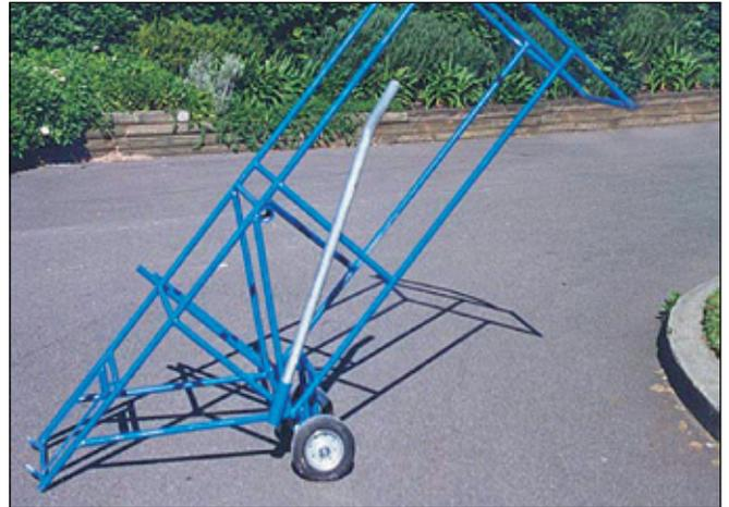
Figure 4.2.2 Hebel Hoist
