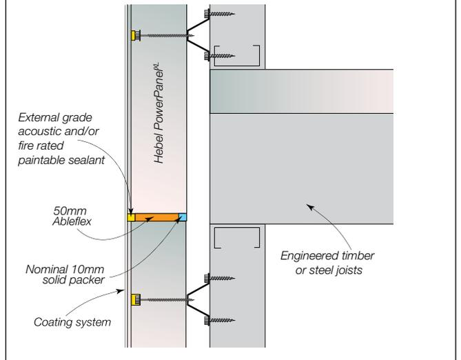
**Figure 3.5.7.7 Horizontal control joint – cavity brickwork to Hebel PowerPanel<sup>XL</sup>**
