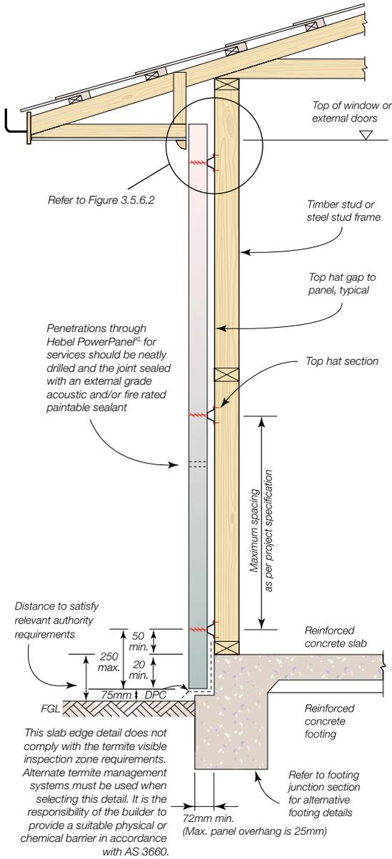
Figure 3.5.1.6 Single storey construction – high wall section detail (3900mm max.)
