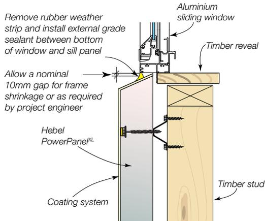
NOTE: Include suitable backing rod and sealant for 5-10mm gaps.
