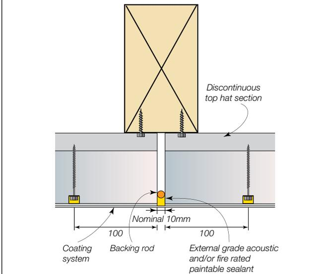
**Figure 3.5.7.10 – Typical vertical control joint with double studs**
