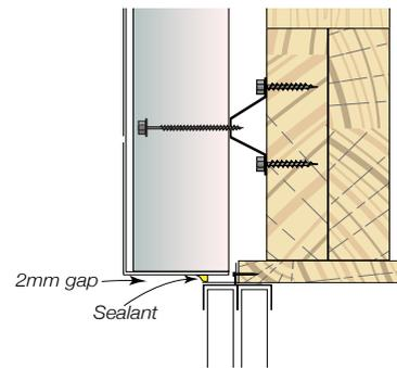
NOTE: Drainage of window and door sills, in either aluminium or timber, should be directed to the outside of the building, on top of the window sill.
