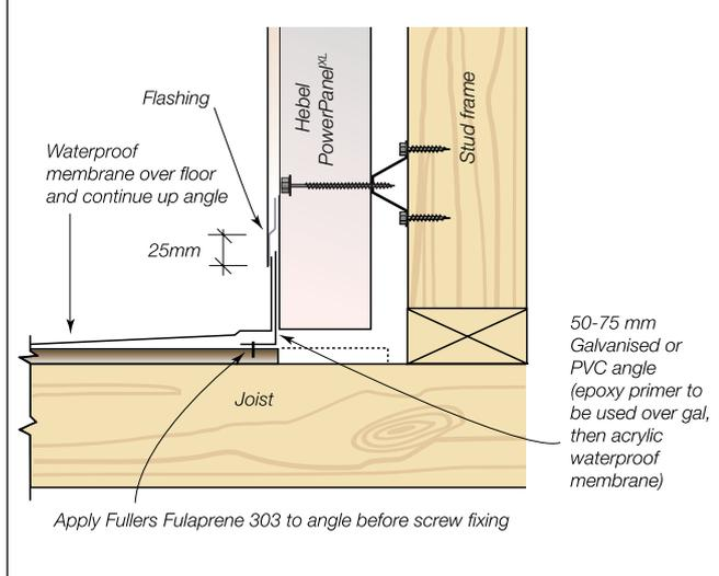
Figure 3.5.6.6 Parapet capping
