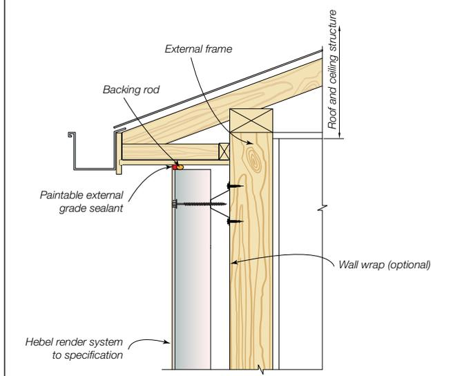
Figure 3.5.6.2 Typical roof eaves detail - Option 2
