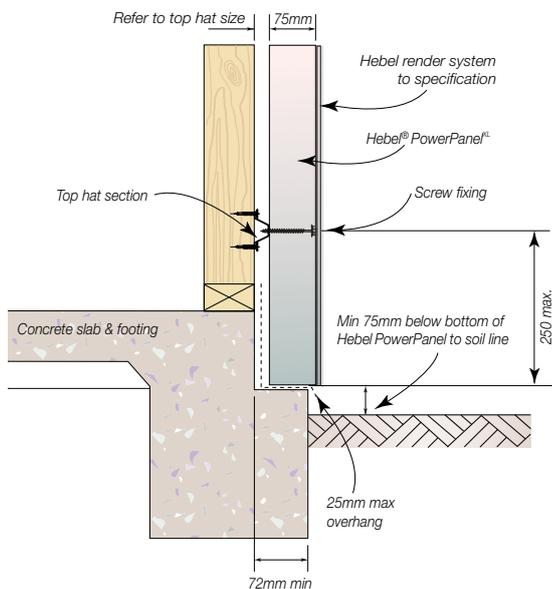
Figure 3.5.5.7 Base detail suspended floor – pier connection
