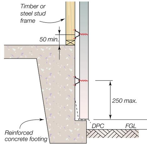
Figure 3.5.5.3 Junction to masonry earth retaining wall
