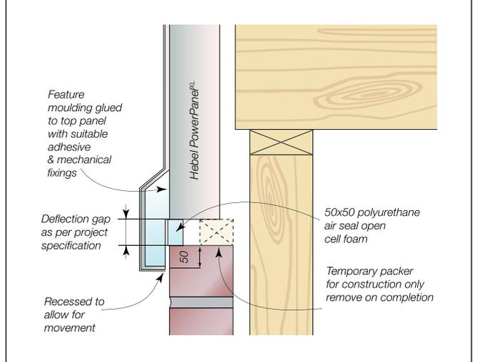
**Figure 3.5.7.9 Typical vertical control joint**
