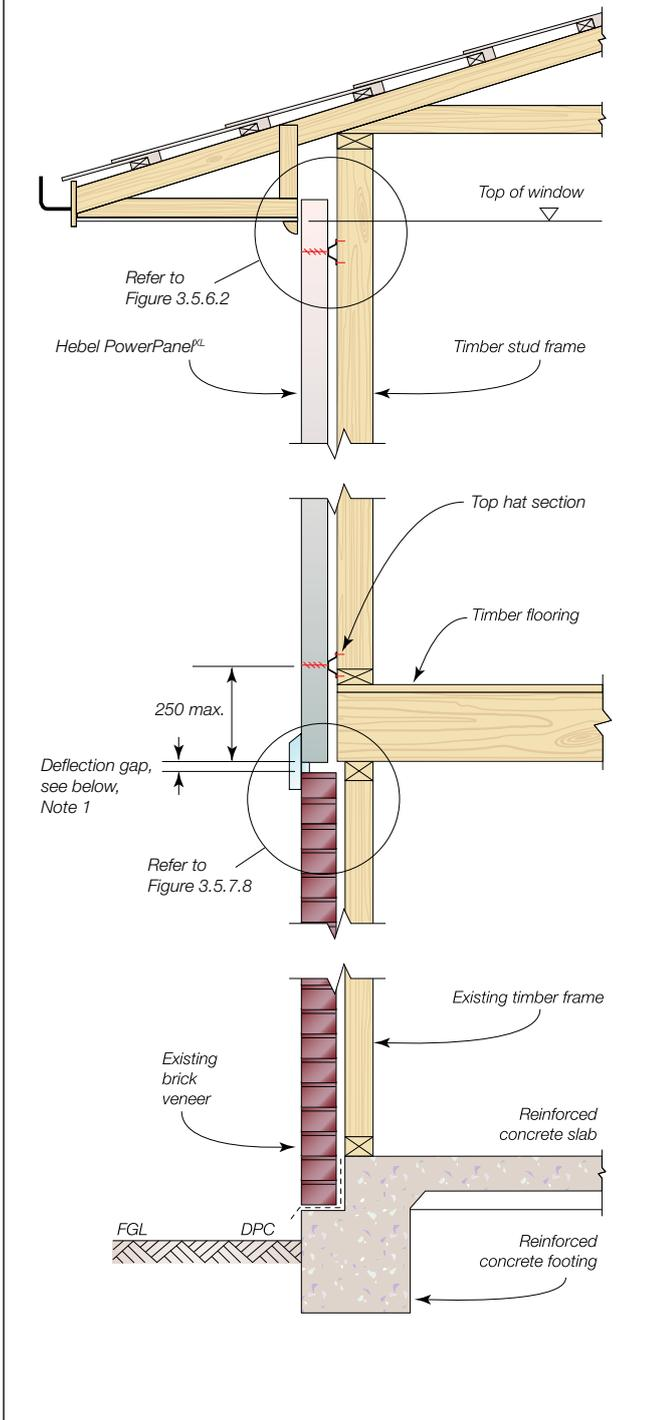
Figure 3.5.3.3 Two storey additions – typical section with double brick below
