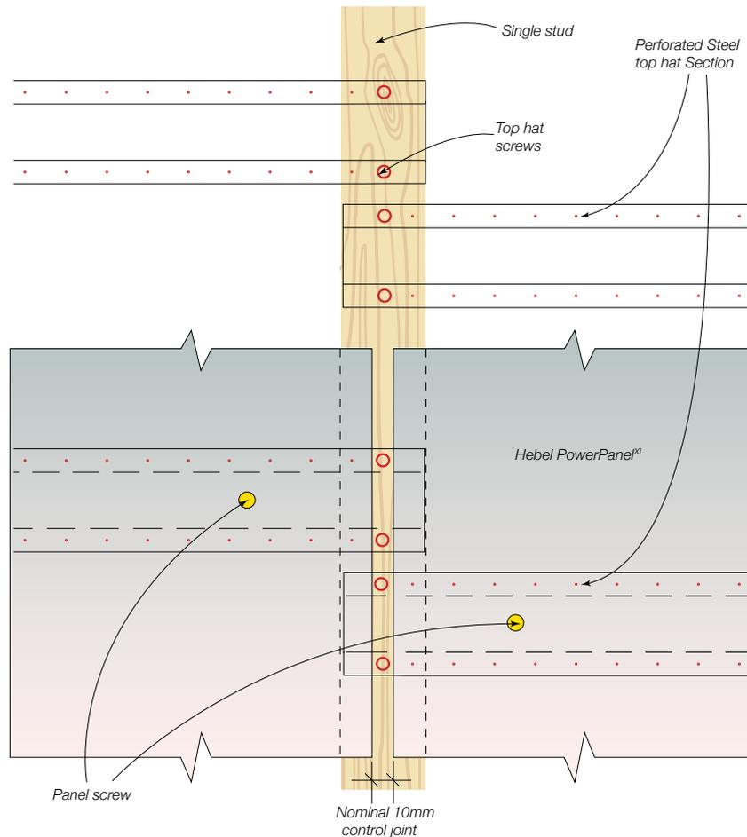
Figure 3.5.7.12 – Typical window control joint detail – lintel over
