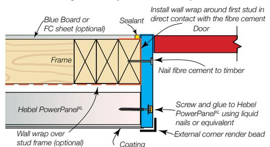
Figure 3.5.8.8 Sliding door sill detail – Option 1 – Concrete sill < 270mm
