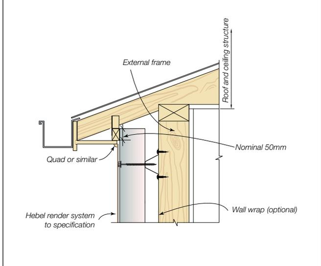
Figure 3.5.6.3 Roof to wall junction detail - Option 1
