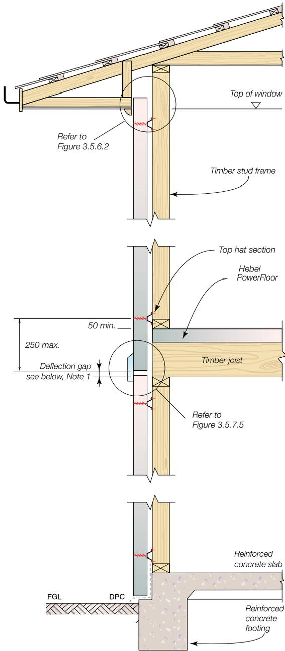
Figure 3.5.2.5 two storey construction – steel frame section or engineered joists with  $\leq 1\%$  shrinkage
