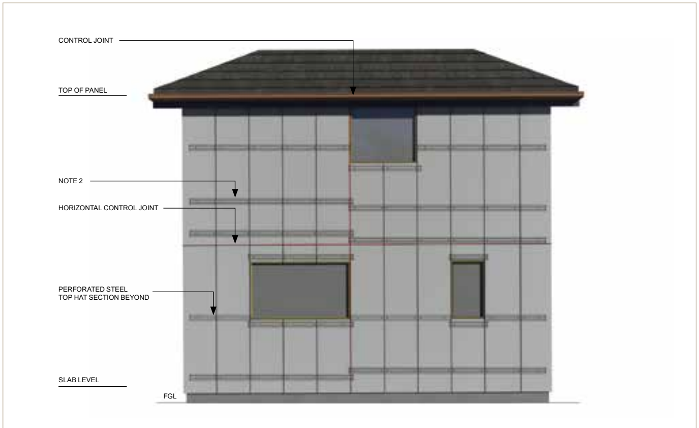
Detail 3.8 – Two storey construction – hip roof elevation
