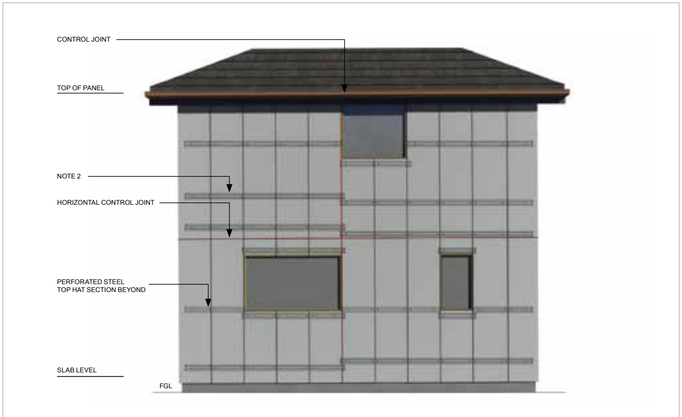
Detail 3.8 – Two storey construction – hip roof elevation
